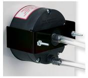
Mounting hardware is supplied with the Minihelic® II gage for panel mounting through a single hole, 2-5/8" (67 mm) in diameter. Panel thickness up to 1/2" (13 mm) can be accommodated with the hardware supplied. If necessary, surface mounting of the gage can be accomplished by means of two 4-40 screws into the tapped mounting bracket stud holes in the rear of the gage. Surface mounting requires clearance holes in the panel for the two pressure taps.
