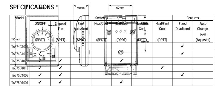
Setpoint range : 10...30°C. By means of a large setpoint
