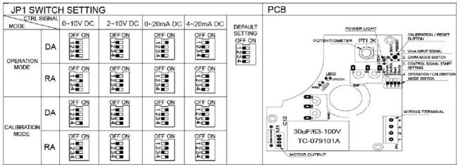
NOTE: we strongly recommend that JP1 switch should be set on operation mode in normal use.
