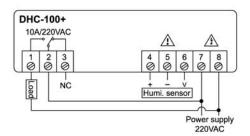
The red wire is "+",which is to connect terminal 4; The black wire is "-",which is to connect terminal 5; The yellow wire is "V", which is to connect terminal 6.
