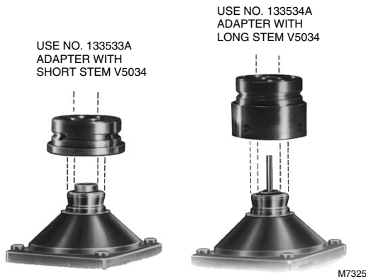
Fig. 3. Use adapters to connect V4055 Actuator with V5034 Valve.
