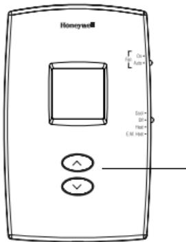
Press the ▲ or ▼ button once to display the setpoint temperature. Press either button more than once to change the setpoint.
