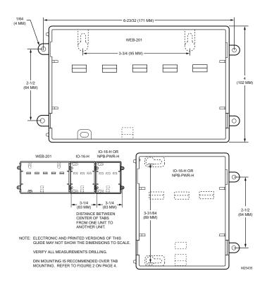
Fig. 1. Tab Mounting Dimensions in Inches (mm).
