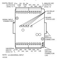
Fig. 3. IO-16-H Wiring Terminal Locations.
